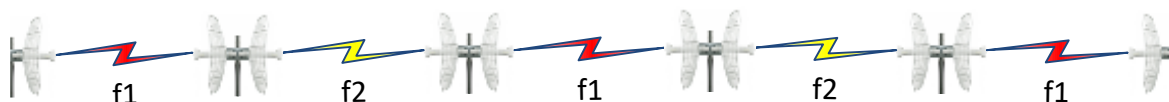
Figure 1 Data Pipeline showing the operation at alternating frequencies on every hop. The MagiNodes are connected back-to-back using their Ethernet ports.
